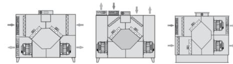
Available with horizontal or vertical duct connection and as outdoor unit
